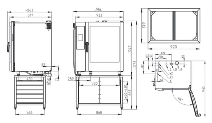
A - Flap valve, B - Chimney, C - Waste connection, E - Electricity, V1 - Untreated water, V2 - Treated water
