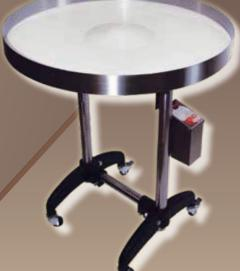
The truffle table is used to coat chocolate pralines with grain, cocoa, coconut powder, etc...
