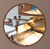
• The air flow device (necessary for the truffles enrobing) can be positioned by using some simple hooks.
